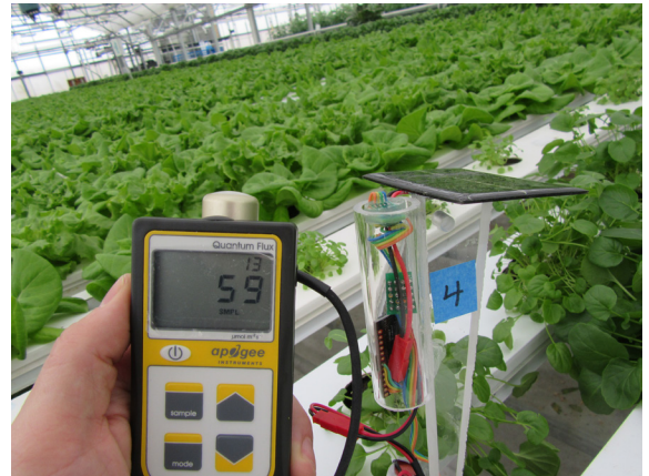
The first prototype light sensors were measured for accuracy against the Apogee Quantum Flux handheld PAR sensor unit.
